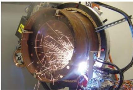
BMT and partners are working to develop, test, and validate a "field ready" HLAW system for full circumferential girth welding of large diameter, high strength steel pipe. Two system designs are being developed (robotic and direct clamp-on platforms) for applications that include both double jointing operations in pipe mills and onshore & offshore pipeline construction projects.
